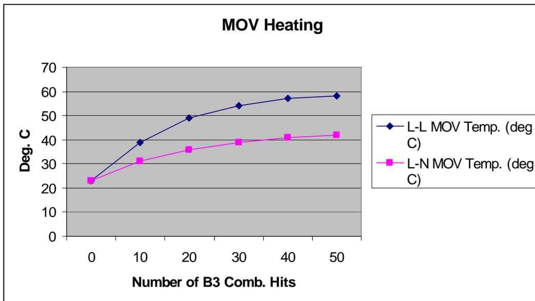
Note that the temperature rise is much higher in the discrete or directly connected 320 V MOV (connected directly from Phase A to Phase B) even though it has a higher maximum operating voltage than the combination of 150 V MOVs in the Phase A to Neutral and the Phase B to Neutral MOVs (300 V total).
