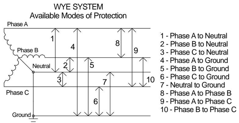
Transient voltage surge suppressors (TVSS) or surge protective devices (SPD) are available in a number of designs with regard to the number of modes protected. Most commonly, these devices offer three, four, seven or ten modes of protection. These configurations are shown in the figures below (a varistor symbol is used to represent a direct or discrete mode of protection).
