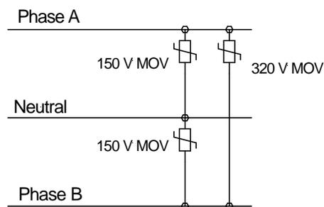
Note that 150 V MOVs are used in the connection from Phase A to Neutral and from Phase B to Neutral and that a 320 V MOV is used in the connection from Phase A to Phase B. This arrangement makes the voltage of the Phase A to Neutral to Phase B combination of MOVs have a maximum operating voltage of 300 V while the directly connected MOV from Phase A to Phase B has a maximum operating voltage of 320 V.
