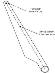
Fig.8. Zone blade conductor retrofit
