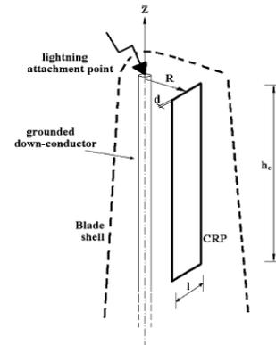
Fig 9. Geometry for the evaluation of eddy currents in a CRP laminate (Adapted from [7] \_2010 IEEE)
