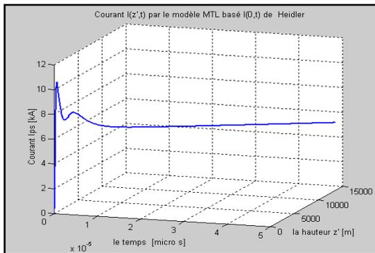
Fig. 5. Current in lightning channel of the Model MTLE with  $(0, t)$  of Heidler
