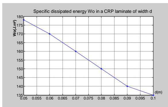
Fig. 10 . Specific dissipated energy in a CRP laminate of width d. (Adapted from [7] \_2010 IEEE)
