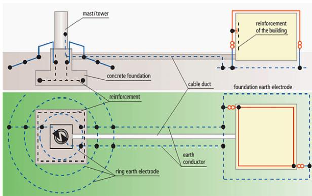
Fig.7. Earthing system with the largest surface of Wind turbine
