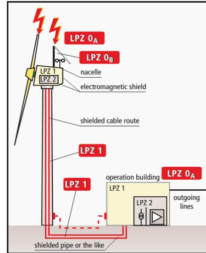
Fig 6. Lightning protection zones concept for a wind turbine
